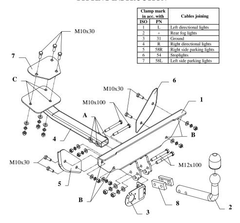
This towbar is designed to assembly in following cars: **FIAT PUNTO, 3-5 doors,** produced since 1994 till 08.1999, catalogue no. **R07** and is prepared to tow trailers max total weight **1300 kg** and max vertical load **50 kg**.
